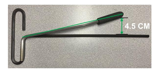
6. Optional - to create black foam tip, buy closed cell 1/2" dowel from Hobby Store, cut to length, drill center hole and sand to shape.
