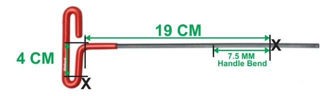
4. Optional "handle" bend: With short end pointing down, heat and bend 7.5mm from long end to 10 0'clock angle, creating 14 MM space from baseline.
